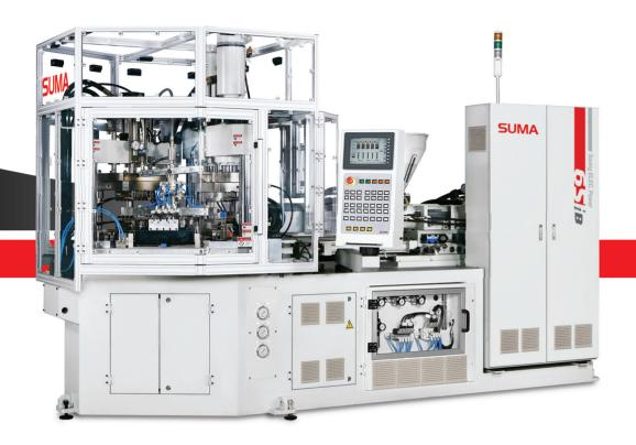
Injection Blow Molding Machinery
