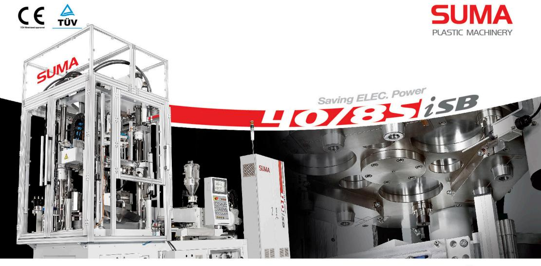
Injection Stretch Blow Molding Machine 3-station
